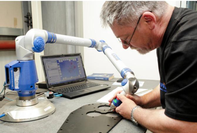
Part measurement with the FARO arm
