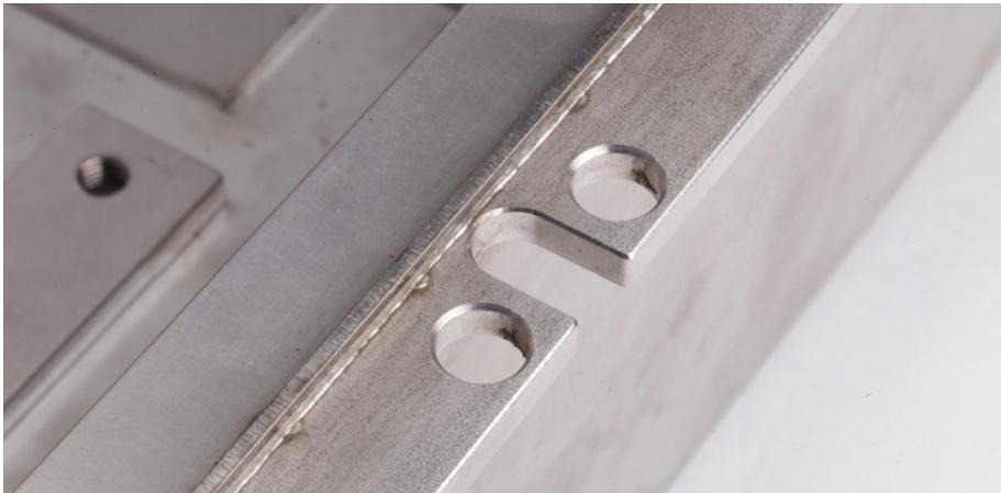
Detailed view of a laser welded seam
